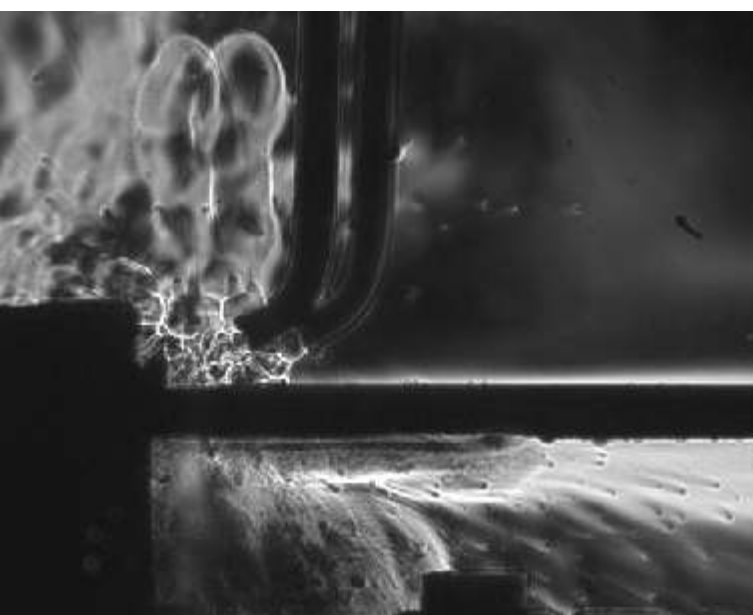
Schlieren image of a laser welding process
